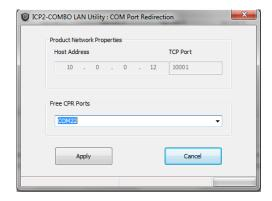
Select desired COM port number and press "Apply". COM Ports list on "COM Port Redirection" window will refresh automatically:
