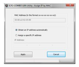
Enter MAC address manually according to sticker printed on the ICP2-COMBO chassis
